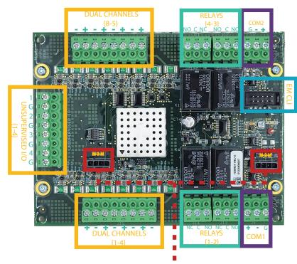
Module to Module Connectors (12VDC @ 4A + Comms) Use P/N 367691186
